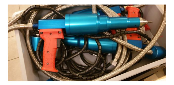
pact Treatment is used in areas of stress concern, or in areas identified as having residual stresses, then fatigue and fatigue cracking can be prolonged or completely avoided. The treatment is so effective that it could extend the service life of any full penetration weld configuration by at least
